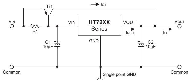
$$R_1 = \frac{V_{BE1}}{I_{REG} \cdot \frac{I_{C1}}{(1+\beta)}} ,$$
