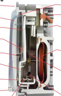
**O-ring seal** for cover assures pressure integrity of case.
