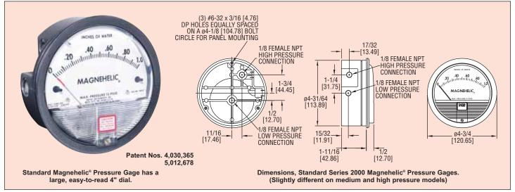
Select the Dwyer® Magnehelic® gage for high accuracy – guaranteed within 2% of full scale - and for the wide choice of 81 models available to suit your needs precisely. Using Dwyer's simple, frictionless Magnehelic® gage movement, it quickly indicates low air or non-corrosive gas pressures - either positive, negative (vacuum) or differential. The design resists shock, vibration and over-pressures. No manometer fluid to evaporate, freeze or cause toxic or leveling problems. It's inexpensive, too.
