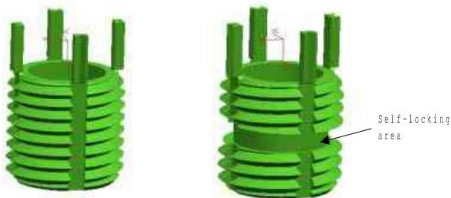
(a) Insert, screw thread, keylocked
