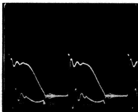
照片 2-4  $V_{DS}$ 及緩衝電容的電流波形 [ $V_{IN}$ =DC125V,  $I_o$ =15A(5V), CH<sub>1</sub>: 100V/div, 2μs/div]
