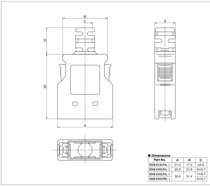
For use with connectors: HDR series IDC type cable connectors HDR-E( )MAG1, HDR-E( )FAG1
