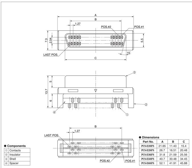
Mating connectors: PCS-E series of DIP type male connectors for PCBs
