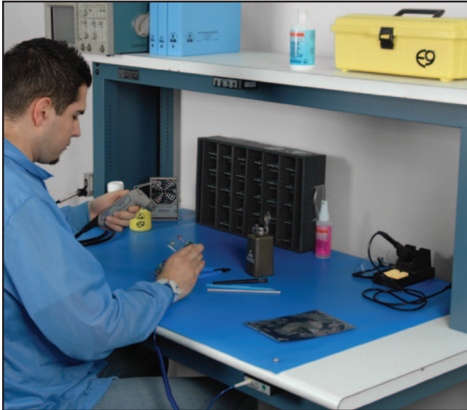
Figure 8: Using the Chargebuster Ion Gun
