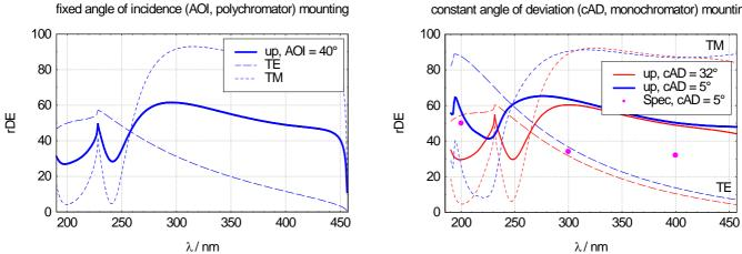
Typical efficiency curves based on rigorous electromagnetic modeling using measured AFM profiles. rDE refers to the ratio between diffracted power from the grating and reflected power from a mirror coated with the same material.
