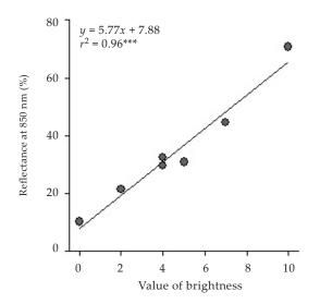
Figure 3. Relation between reflection values of soils at 850 nm measured with laboratory configuration OMK and rating of soil brightness (n = 20, \*\*\* indicates significance at the P < 0.001 level)
