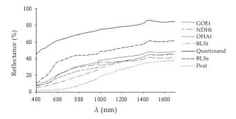
Figure 1. Soil reflectance at different wavelengths ( $\lambda$ ) measured with laboratory config $\lambda$ uration OMK as affected by soil type and origin (n = 20)
