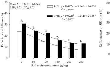
Figure 5. Reflection values at 850 nm of two different agricultural soils (S): Bad Lauchstaedt (white) and Nordhausen (black) as affected by varied soil moisture contents (M) measured with laboratory configuration OMK (means followed by different letters are significantly different at P < 0.05, Tukey, n = 20) and relations between reflectance at 850 nm and soil moisture content (n = 20, \*\*\* indicates significance at the P < 0.001 level)
