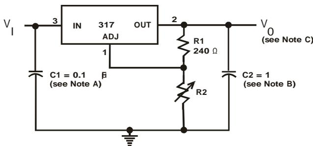
Note A: Use of an input bypass capacitor is recommended if regulator is far from filter capacitors.
