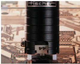
Measurement probe ERCU N for small measurement areas
