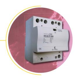
DS60PV are Type 1 Heavy Duty Surge Protectors are designed to protect against lightning surge voltages in photovoltaic power supply networks. These units must be installed in parallel on the DC networks to be protected and provide common mode protection. These protectors are recommended when a direct lightning strike is possible on the installation.
