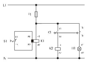
When the contact S1 opens, K2 energizes immediately and the light H1 goes off. After completion of the selected timing K2 returns to its rest position and the light H1 comes on.
