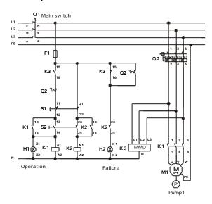
The MMU monitors the pump motor for over voltage.
