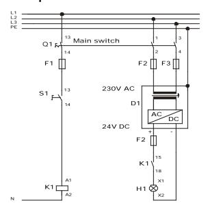
The SKR coupling relay electrically isolates an input signal from an output signal.
