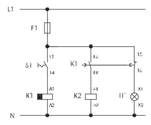
When the contact S1 closes, K2 energizes immediately and the light H1 goes off. Upon completion of the selected timing period K1 returns to its rest position and the light H1 comes on.
