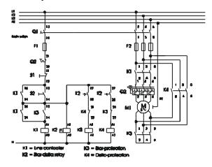
After actuation of element S2, the timing cycle begins.
