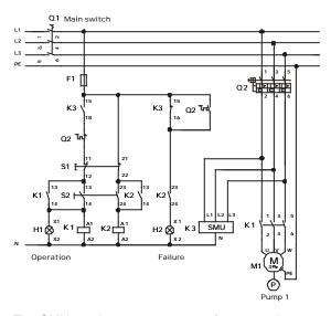
The SMU monitors a pump motor for over voltage.
