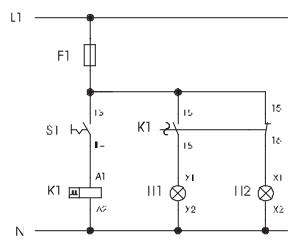
When the contact S1 closes, the lights H1 and H2 blink alternately to the selected timing cycle (H1 begins with pause).
