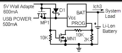
Fig.5:Combining Wall Adapter and USB Power
