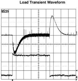
VIN=3.3<sup>1</sup>V, Vout=12V, Iout=5mA->50mA->5mA L=10μH, Cout=4.7μF+0.1μF, Cff=560pF CH1:Vout, 100mV/DIV, Time=1ms/DIV CH4:Iout, 20mA/DIV
