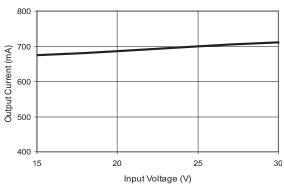
Output Current vs Input Voltage (3 LEDs)
