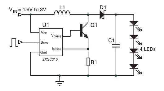
Figure 1 Schematic diagram
