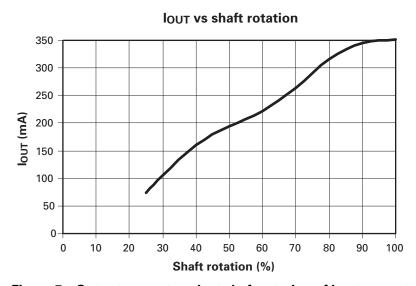
Figure 7 Output current against shaft rotation of log type pot
