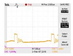
5.5V input with an 18mA load producing 28V DC output
