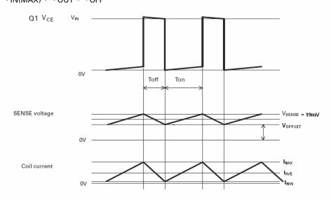
Figure 2 Example of current and voltage waveforms for circuit using ZXSC300 with feed forward network
