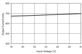
Output Current vs Input Voltage (4 LEDs)
