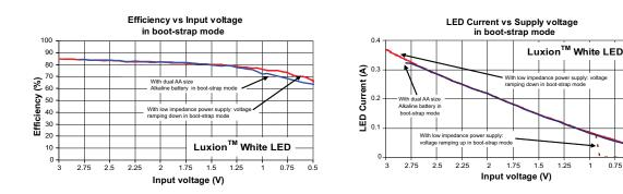
Figure 6 Efficiency vs. input supply voltage Figure 7 LED current vs. input supply voltage
