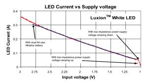
Figure 4 Efficiency vs. input signal voltage Figure 5 LED current vs. input supply voltage
