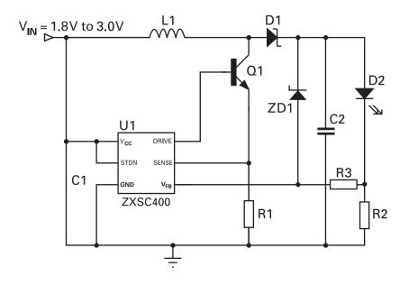
Figure 3 Open circuit protection
