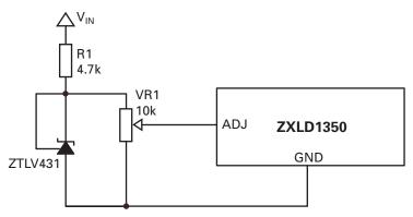
Figure 5 Typical circuit of DC voltage dimming
