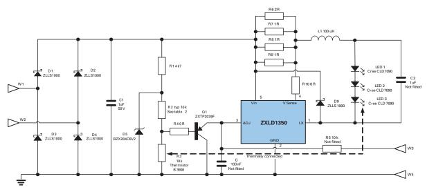
Figure 2 Circuit diagram of ZXLD1350 MR16 lamp solution
