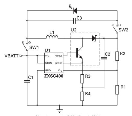
Charging mode: SW1 closed, SW2 open Discharging mode: SW1 open, SW2 closed
