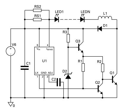
Figure 1 Schematic of 700mA driver
