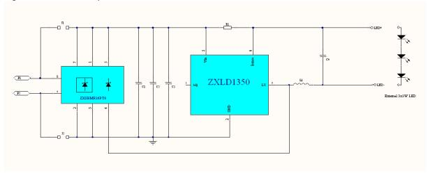
Figure 2 System diagram of ZXLD1350 MR16 Lamp Solution
