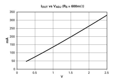
Figure 3 Typical output current versus ADJ voltage with  $R_S = 600 \text{m}\Omega$
