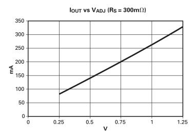
Figure 1 Typical output current versus ADJ voltage with  $R_S$  = 300m $\Omega$
