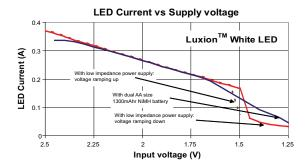
Figure 2 Efficency vs. input supply voltage Figure 3 LED current vs. input supply voltage
