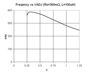
Figure 2 Typical switching frequency versus ADJ voltage with R  $_{S}$  = 300m  $\Omega_{r}$  L=100  $\mu$ H
