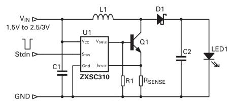
Figure 1 Typical dual cell battery powered 1W LED drive circuit
