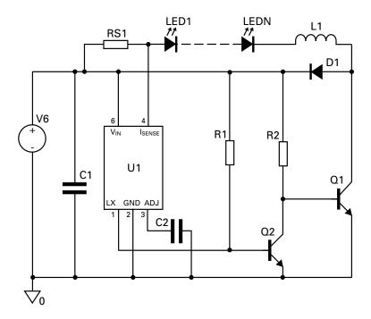
Figure 2 Schematic of 1A driver
