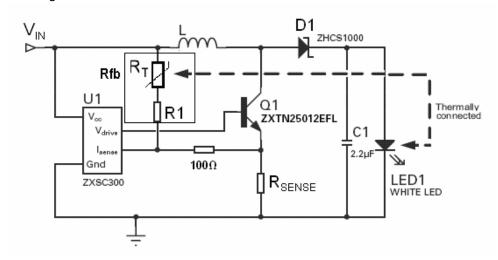
Figure 1 Circuit diagram of ZXSC300 with feed forward and thermal compensation
