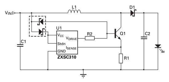
Figure 4 LED flashlight application without bootstrap
