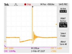
At 5.5V input and an output of 28V, this graph shows the typical output regulation to be <10% and ripple <1V from no load to full load.
