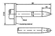
The Unjointed/rigid Finger Probe is made for forceful insertion where the flexibility of the Jointed Finger Probe would be a hindrance. The UFP-01 meets IEC 60950 and 61010, CSA and UL requirements. This probe is precision made of flash chrome plated steel and the rest of the instrument of Delrin®. The handle can be threaded for use with our digital force gauges.
