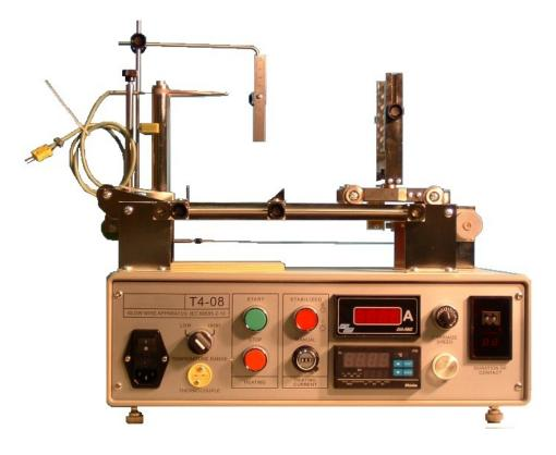
T4-08 GLOW WIRE TEST APPARATUS WITH MOTOR DRIVE is intended for testing the flammability and ignitability of components and materials. It is constructed in compliance with IEC (e.g 60695-2-10, 695-2-1, 335-1, 1058-1, 742, 669-1,) and also includes electronic feed back heating current stabilizer - regulator, A-meter, thermometer, motor drive and timer.
