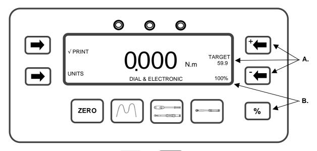
A. To change the limit target value, use target value set is shown on the display. Keep either key depressed for fast target value change.
