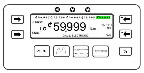
The Professional Torque Tester (Pro-Test) has been designed as an accurate, cost effective and easy to operate instrument for calibrating and testing all types of torque wrenches.
