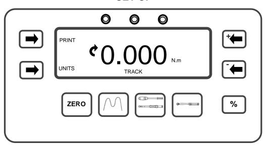
To enter SET UP, press 'UNITS' & 'PRINT' buttons simultaneously upon which the 'SOFTWARE VERSION NUMBER' will be displayed for 2 seconds.
