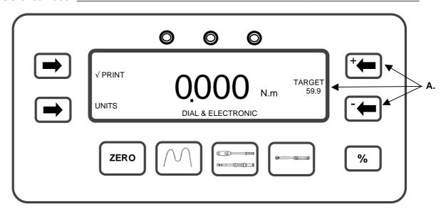
NON ISO 6789:2003 limit mode allows the user to set upper and lower limits from 0% to 99% of the target value.
