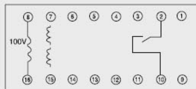
BDZ-1B型内部接线图 Type internal wiring diagram
