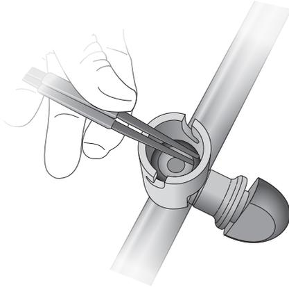
4. Clean the O-ring and the filtration head support using a nonwoven wipe moistened with one of the products listed in the recommended cleaning agents list in this section.
