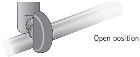
8. When the filtration is finished, rotate the valve button clockwise to the end stop.
