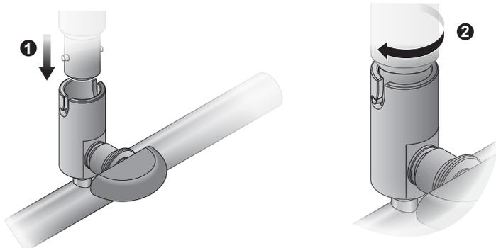
3. Place the filtration device on the filtration head.
