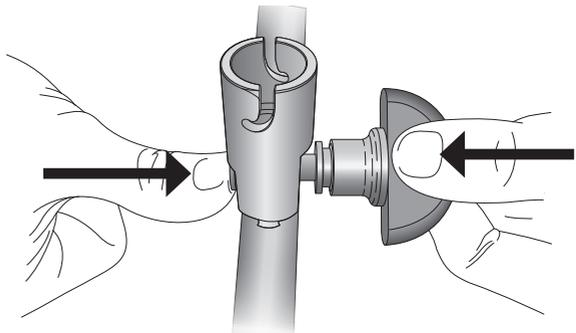
16. Actuate the valve button to check that it is properly assembled. Then, rotate the valve button clockwise to the end stop (closed position).
