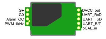
Figure 2. Pin assignment
