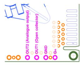
Figure 3. Senseair K33 ICB OBA side) (G+, GND, OUT1 and OUT2, 5.08mm hole spacing
