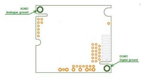
Figure 5. Senseair K33 ICB ground / shield attachment
