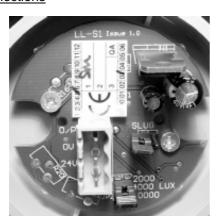
24V = Supply 0v = GndO/P = 0-10Vdc output
