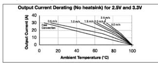
The graph above shows the allowable maximum output current to maintain a maximum  $+100^{\circ}$ C case temperature. Note that the ambient temperature is the air temperature adjacent to the power module which is typically elevated above the room environmental temperature.
