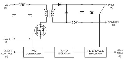
Figure 1. Simplified Schematic
