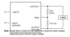
Figure 4. Trim Connections Using Fixed Resistors
