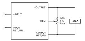
Figure 3. Trim Connections Using a Trimpot
