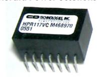
The HPR1XXVC Series uses advanced circuit design and packaging technology to deliver superior reliability and performance. A 170kHz push-pull oscillator is used in the input stage. Beatfrequency oscillation problems are reduced when using the HPR1XXVC Series with high frequency isolation amplifiers.
