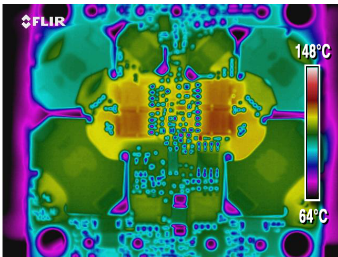
Figure 10. Thermal Image, Bottom View (VIN = 48V, TA = +25°C, IOUT = 14.1 Amps, natural convection, unmounted)
