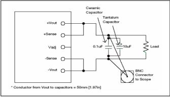
Output ripple and noise test setup
