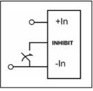
The products are equipped with a Inhibit control function referenced to the primary negative input connection (- In), positive logic. The INHIBIT function allows the regulator to be turned on/off by an external device like a semiconductor or mechanical switch.
