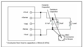
Output ripple and noise test setup
