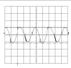
Output voltage ripple (50mV/div.) at  $T_{Pcb}$ =+25 °C, Vin=53 V, Io=6.67A resistive load with C=10 µF tantalum and 0.1 µF ceramic capacitors. Band width=20MHz. Time scale: 1µs / div.
