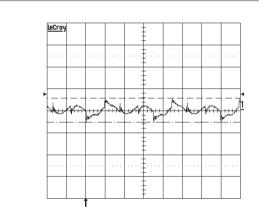
Output voltage ripple (100mV/div.) at T<sub>Pcb</sub>=+25 °C, Vin=53 V, Io=20A resistive load with C=10  $\mu F$  tantalum and 0.1  $\mu F$  ceramic capacitors. Band width=20MHz. Time scale: 2 $\mu s$  / div.
