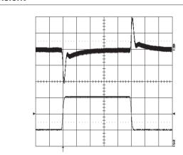
Output voltage response to load current step-change (2.0-6.2-2.0 A) at  $T_{Pcb}$ =+25 °C, Vin=53 V. Top trace: output voltage (200mV/div.). Bottom trace: load current (2 A/div.) Time scale: 0.1 ms/div.
