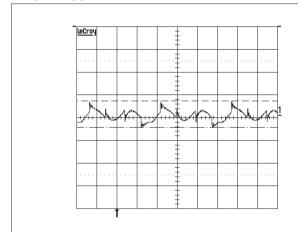
Output voltage ripple (100mV/div.) at T<sub>Pcb</sub>=+25 °C, Vin=53 V, Io=25A resistive load with C=10 μF tantalum and 0.1 μF ceramic capacitors. Band width=20MHz. Time scale: 2µs / div.
