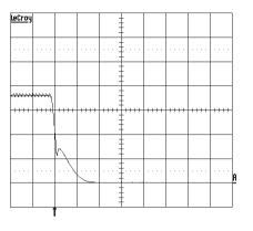
Turn-off at Io=10A resistive load at T<sub>Pcb</sub>=+25 °C, Vin=53 V. Turn-off enabled by disconnecting Vin. Output voltage (0.50 V/div.). Time scale: 50 µs/div.
