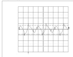
Output voltage ripple (100mV/div.) at T<sub>Pcb</sub>=+25 °C, Vin=53 V, Io=30A resistive load with C=10  $\mu F$  tantalum and 0.1  $\mu F$  ceramic capacitors. Band width=20MHz. Time scale: 2 $\mu s$  / div.
