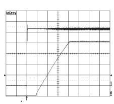
Start-up at Io=30A resistive load at  $T_{Pcb}$ =+25 °C, Vin=53 V. Start enabled by connecting Vin. Top trace: input voltage (10 V/div.). Bottom trace: output voltage (1 V/div.). Time scale: 5 ms/div.
