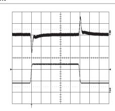
Output voltage response to load current step-change (1.7-5.0-1.7 A) at  $T_{Pcb}{=}+25~^{\circ}C,\ Vin{=}53~V.$  Top trace: output voltage (200mV/div.). Bottom trace: load current (2 A/div.) Time scale: 0.1 ms/div.
