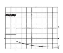
Turn-off at lo=25A resistive load at T $_{Pcb}$ =+25 °C, Vin=53 V. Turn-off enabled by disconnecting Vin. Top trace: output voltage (2 V/div.). Bottom trace: input voltage (20 V/div.). Time scale: 10 ms/div.
