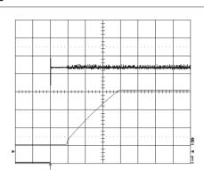
Start-up at Io=6.67A resistive load at  $T_{Pcb}$ =+25 °C, Vin=53 V. Start enabled by connecting Vin. Top trace: input voltage (10 V/div.). Bottom trace: output voltage (5 V/div.). Time scale: 5 ms/div.
