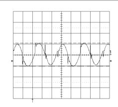
Output voltage ripple (100mV/div.) at  $T_{Pcb}$ =+25 °C, Vin=53 V, Io=8.33A resistive load with C=10 µF tantalum and 0.1 µF ceramic capacitors. Band width=20MHz. Time scale: 1µs / div.
