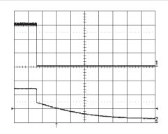
Turn-off at lo=6.67A resistive load at  $T_{Pcb}$ =+25 °C, Vin=53 V. Turn-off enabled by disconnecting Vin. Top trace: output voltage (5 V/div.). Bottom trace: input voltage (20 V/div.). Time scale: 10 ms/div.
