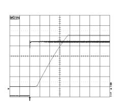
Start-up at lo=20A resistive load at  $T_{Pcb}$ =+25 °C, Vin=53 V. Start enabled by connecting Vin. Top trace: input voltage (10 V/div.). Bottom trace: output voltage (1 V/div.). Time scale: 5 ms/div.
