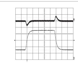
Output voltage response to load current step-change (7.5-22.5-7.5 A) at  $T_{Pcb}$ =+25 °C, Vin=53 V. Top trace: output voltage (200mV/div.). Bottom trace: load current (5 A/div.) Time scale: 0.1 ms/div.
