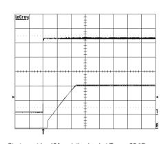
Start-up at lo=40A resistive load at  $T_{Pcb}$ =+25 °C, Vin=53 V. Start enabled by connecting Vin. Top trace: input voltage (10 V/div.). Bottom trace: output voltage (0.50 V/div.). Time scale: 10 ms/div.
