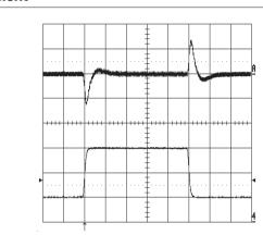
Output voltage response to load current step-change (5.0-15-5.0 A) at  $T_{Pcb}$ =+25 °C, Vin=53 V. Top trace: output voltage (200mV/div.). Bottom trace: load current (5 A/div.) Time scale: 0.1 ms/div.
