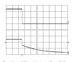
Turn-off at Io=8.33A resistive load at  $T_{Pcb}$ =+25 °C, Vin=53 V. Turn-off enabled by disconnecting Vin. Top trace: output voltage (5 V/div.). Bottom trace: input voltage (20 V/div.). Time scale: 10 ms/div.
