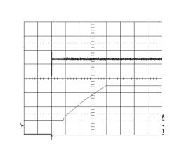
Start-up at Io=8.33A resistive load at  $T_{Pcb}$ =+25 °C, Vin=53 V. Start enabled by connecting Vin. Top trace: input voltage (10 V/div.). Bottom trace: output voltage (5 V/div.). Time scale: 5 ms/div.
