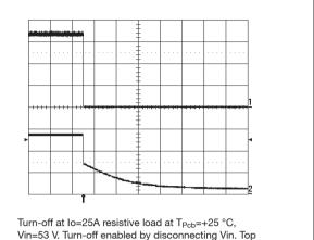
trace: output voltage (1 V/div.). Bottom trace: input voltage (20 V/div.). Time scale: 10 ms/div.
