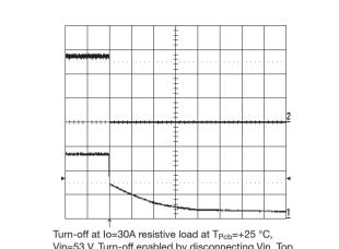
Turn-off at Io=30A resistive load at T<sub>Pcb</sub>=+25 °C, Vin=53 V. Turn-off enabled by disconnecting Vin. Top trace: output voltage (1 V/div.). Bottom trace: input voltage (20 V/div.). Time scale: 10 ms/div.
