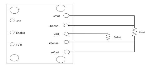
Figure 4. Circuit Configuration to Increase Output Voltage.
