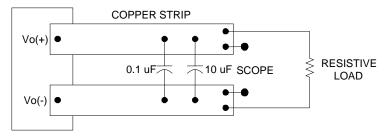
Note: Use a 0.1µF @50V X7R ceramic capacitor and a 10µF @ 25V tantalum capacitor. Scope measurement should be made using a BNC socket. Position the load between 51 mm and 76 mm (2 in. and 3 in.) from module.
