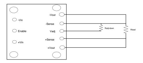
Figure 5. Circuit Configuration to Decrease Output Voltage.
