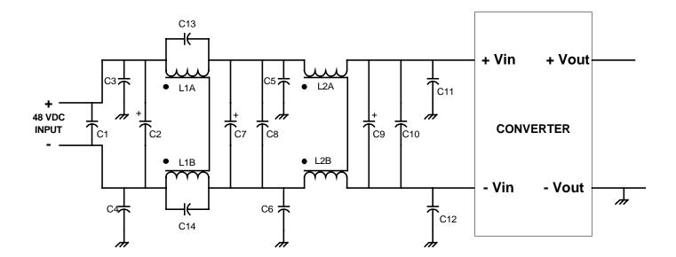
Figure 12: Class B Filter Circuit
