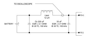
Note: Measure input reflected-ripple current with a simulated source inductance (Ltest) of 12 uH. Capacitor Cs offsets possible battery impedance. Measure current as shown above.
