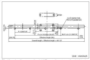
\*Mount the scale on the non-magnetic material. When mounting on a magnetic material, insert a non-magnetic layer with a thickness of at least 3mm.
