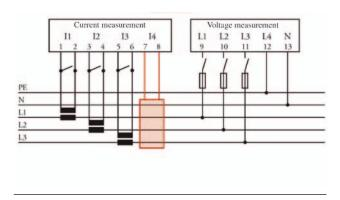
Illustration: Connection for measurement channels and differential current transformer of series KBU (split core).
