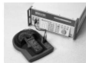
5500A / COIL 选件, 用于钳型表校准
