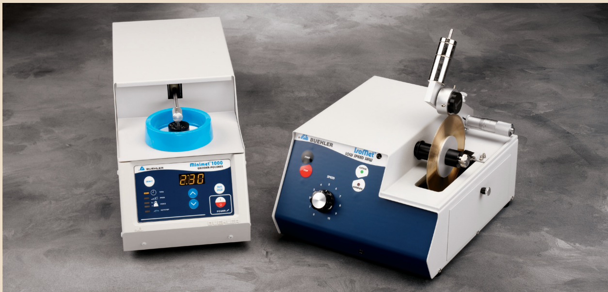
The IsoMet® Low Speed Saw is an excellent companion to the MiniMet® 1000 Grinder/Polisher including when low deformation sectioning is required prior to polishing.
