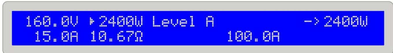
Figure 9. Normal load operation in CP regulation mode
