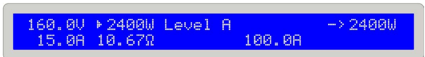
Figure 9. Normal load operation in CP regulation mode
