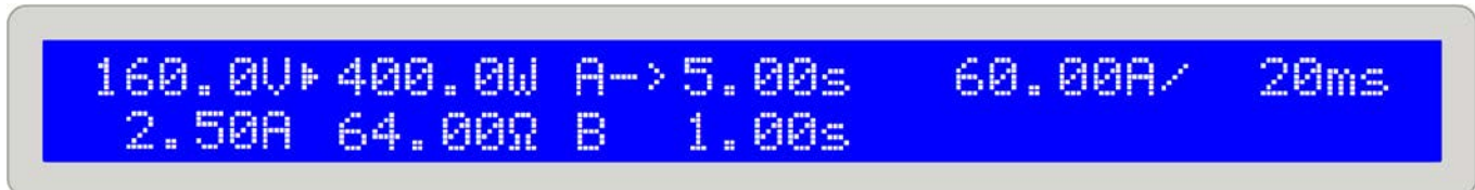
Figure 10. Level A/B operation with pulse width adjustment
