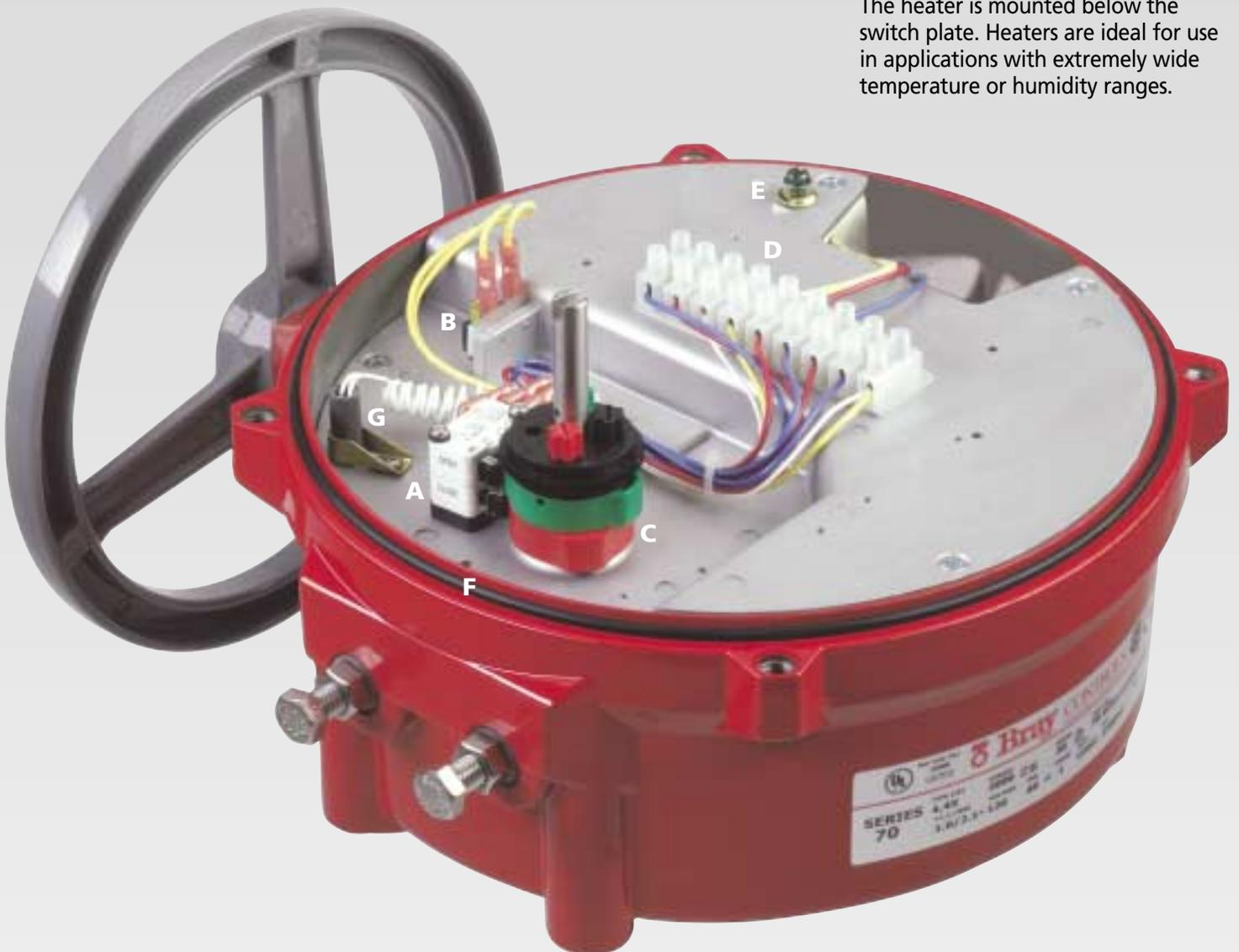
Bray designed the R<sup>4</sup> to completely separate the Control Center from the Power Center. The Power Center, located in the actuator base, consists of motor, gear train, capacitor, output drive and heater. This design protects the power drive system as each component has been engineered to require no customer servicing. The Power Center components have been uniquely configured to maintain the extremely low profile of the R<sup>4</sup>.
