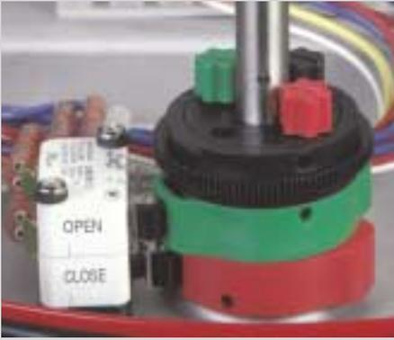
**CAMS / CAM ADJUSTMENT (C)**
