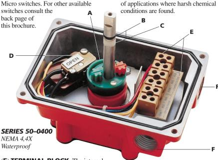
(E) TERMINAL BLOCK The internal switches are pre-wired to a terminal block. The block has been designed for ease of wiring installation with clearly marked wire numbers for both open and closed switches.
