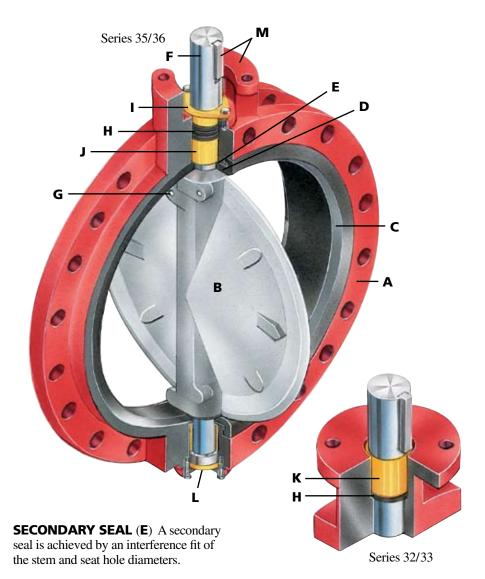
**STEM** (**F**) Bray's one piece through stem design is completely isolated from the flowing media and achieves high torsional strength. The stem ends are standardized for direct mounting and interchangeability with Bray actuators.
