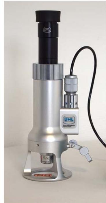
The flexible lamp holder enables an optimal setting of the angular illumination.
