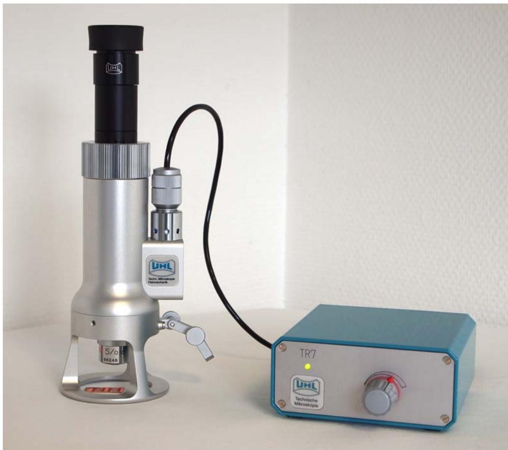
Portable measuring microscope with coaxial and angular incident illumination of high quality.
