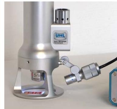
For independent operation from the electric main power, a LED battery lamp is available.
